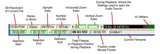
Note that in the above picture, some fields are outlined with a green box. These fields allow you to edit them by clicking into them. For example, you can manually key in a Zoom Ratio and press Enter to instantly zoom to that ratio. You can also adjust your selection by keying in a time using the currently displayed format. See the <a href="Text Entry Fields"><u>Text Entry Fields</u></a> topic for details.
