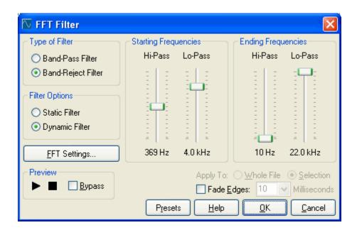
Unlike the <u>Graphic Equalizer</u>, the FFT filtering uses a Fourier Transform to perform filtering. The result is a "brick wall" filtering, where anything beyond the range of the filter is completely filtered out.
