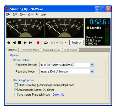
The *Recording Device* allows you to select among your installed sound cards. You can choose any card that is capable of recording.
