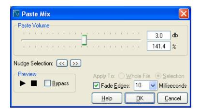
This function lets you mix the Clipboard contents with the current file. You can adjust the audio level of the pasted audio with the Level control.
