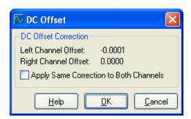
This feature lets you correct a DC offset in a sound file. A DC Offset is where the entire wave is shifted up or down, where zero is not quite zero. Some inexpensive sound cards may record audio with an offset that isn't quite zero; this feature will let you correct this.
