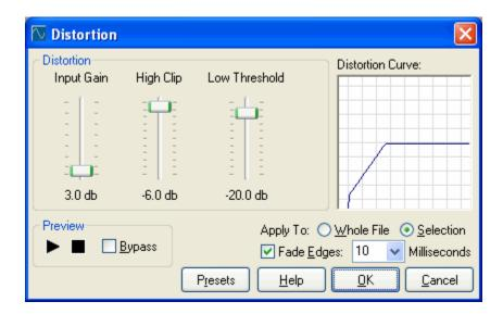
The Distortion processor lets you clip your audio, as well as set a low threshold. Audio above the Clip threshold will be clipped. Audio below the Low threshold will be silent.
