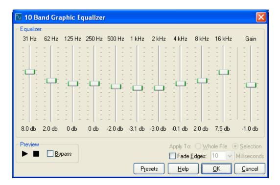
NGWave offers a 10-band Graphic Equalizer. This functions very much like a standard analog equalizer. The code mimics analog circuitry as much as possible, resulting in a very warm equalization.
