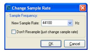
This dialog lets you resample the file to a new sampling rate. NGWave uses a band-limited linear interpolation technique that provides fast and good quality sample rate conversions.
