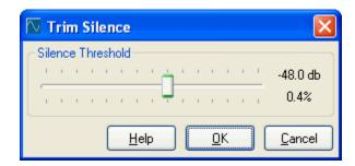
This feature removes leading and trailing silence from the current file. You can select the Threshold for the silence detection; anything below that threshold is considered "silence".
