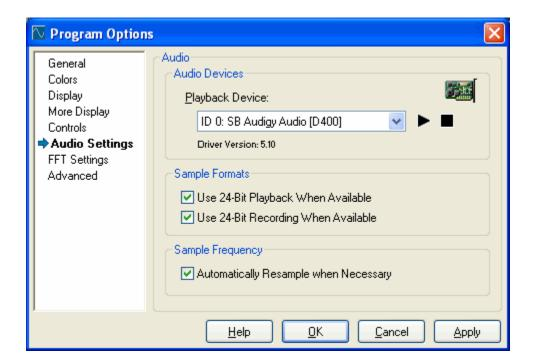
Audio Device - You can select which of your installed sound cards NGWave will play audio through. Use the Play/Stop buttons to play a sound through the selected device. The sound played is a file called "test.mp3", residing in NGWave's program folder. Note that when you select an audio device, its driver version is displayed for reference.
