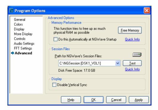
Free Memory - This feature performs an operation similar to Free Mem or RAM Defrag utilities. It simply allocates a large amount of memory, then frees it, forcing Windows to flush unused memory such as the disk cache. The result is faster access to new memory, and a perceived faster response in some programs. Specifically, this can help NGWave if you are experiencing glitches during playback or recording.
