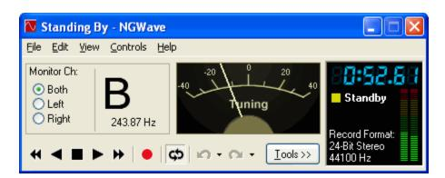
The note displays in a large font so you can see it from a distance. The tuner needle shows how far off the input is from the detected note. The tuner is as accurate as your sound card's clock frequency, typically within a few thousandths of a percent.
