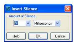
This function simply adds blank audio data, or silence, into the file.
